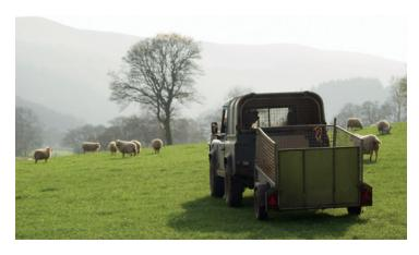
These rules are especially important when carrying livestock. The movement of livestock in transit can't be predicted so it is extremely important to ensure the weight is distributed as evenly as possible by using internal safety gates.
